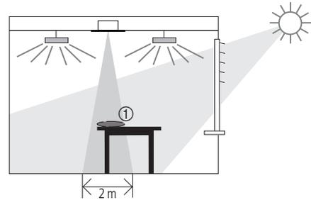
$$\text{Room correction factor} = \frac{\text{Brightness value at the ceiling}}{\text{Brightness value on the work surface}}$$
